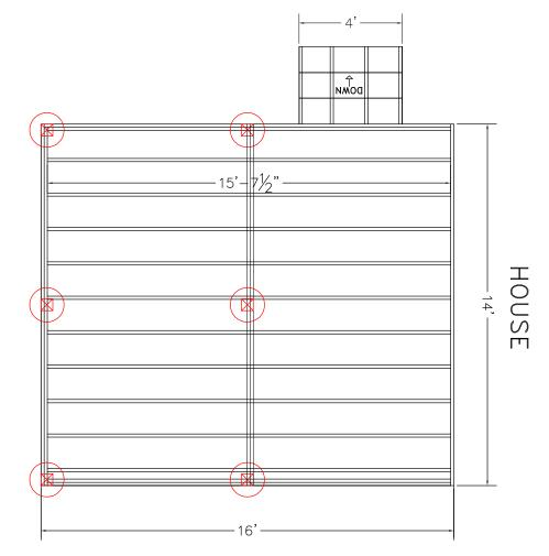
FOOTING SIZES ADJUSTED FOR ADDITIONAL 25 LBS PER SQUARE FOOT SNOW / ROOF LOAD  $(\boxtimes)$
