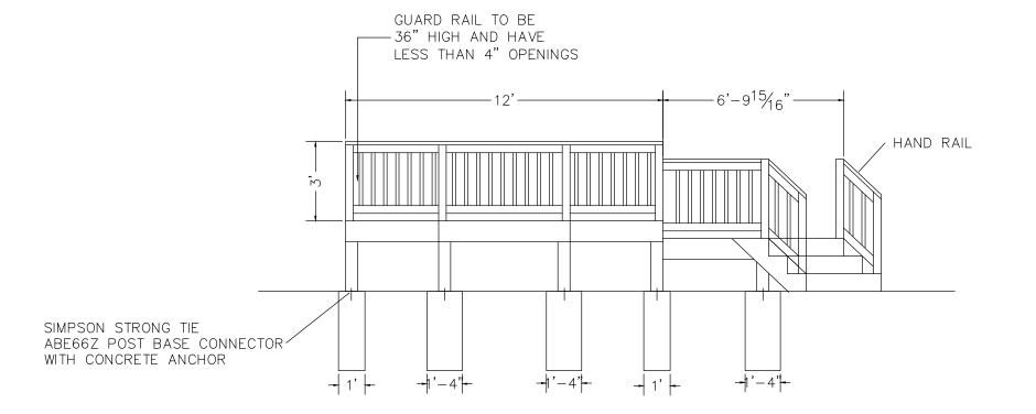
EQUIVALENT FASTENERS ENINGS PER IRC CODE (see rail detail)
