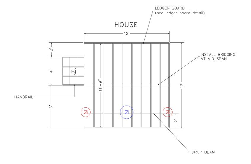
$\sim$ OR EQUIVALENT FASTENERS BOLTS WITH WASHERS LEDGER BOARD TO BE FLASHED AND BOLTED (2 (SEE LEDGER DETAIL IN DECK CONSTRUCTION GI JOISTS TO BE 2x10 SOUTHERN YELLOW PINE TR BEAMS TO BE 2-2x10 SOUTHERN YELLOW PINE RAILS TO BE 36" HIGH WITH LESS THAN 4" OP STAIRS TO BE BUILT MAX RISE 7 3/4" MIN RIS
