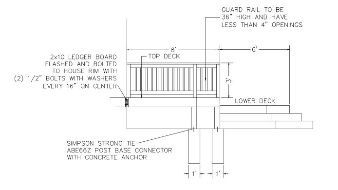
EDGER BOARD TO BE FLASHED AND BOLTED (2) 1/2" BOLTS WITH WASHERS OR EQUIVALENT FASTENER:
