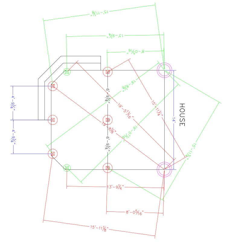
DISCLAIMER: USE ONLY 2,500 PSI CONCRETE FOR FROST FOOTING FOUNDATIONS
