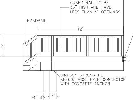
2x10 LEDGER BOARD FLASHED AND BOLTED TO HOUSE RIM WITH (2) 1/2" BOLTS WITH WASHERS EVERY 16" ON CENTER
