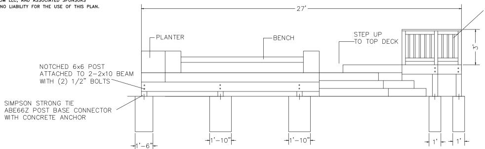
GUARD RAIL TO BE 36" HIGH AND HAVE LESS THAN 4" OPENINGS
