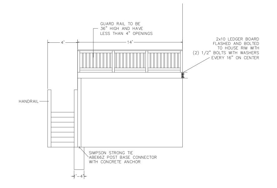
IGER BOARD TO BE FLASHED AND BOLTED (2) 1/2" BOLTS WITH WASHERS OR EQUIVALENT FASTENERS E LEDGER DETAIL IN DECK CONSTRUCTION GUIDE)
