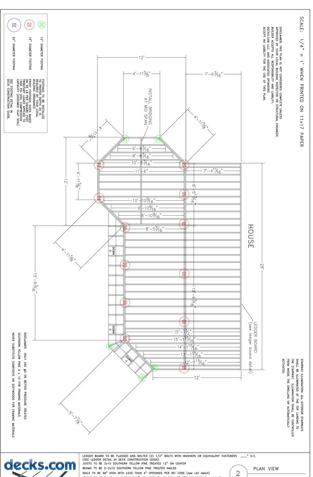
RAILS TO BE 36" HIGH WITH LESS THAN 4" OPENINGS PER IRC CODE (see rail detail) STAIRS TO BE BUILT MAX RISE 7 3/4" MIN RISE 4" MIN RUN 10" PER IRC CODE (see detail)
