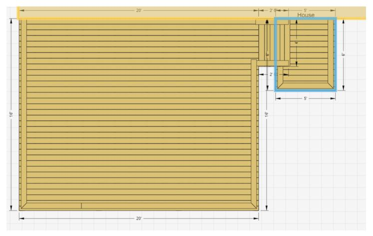
Then add the stairs to the second deck/level. Adjust width if desired.
