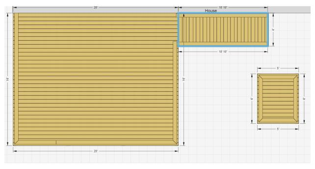
Move the Landing or second deck into position under the stairs when in the right position the stairs will "snap to lower deck.
