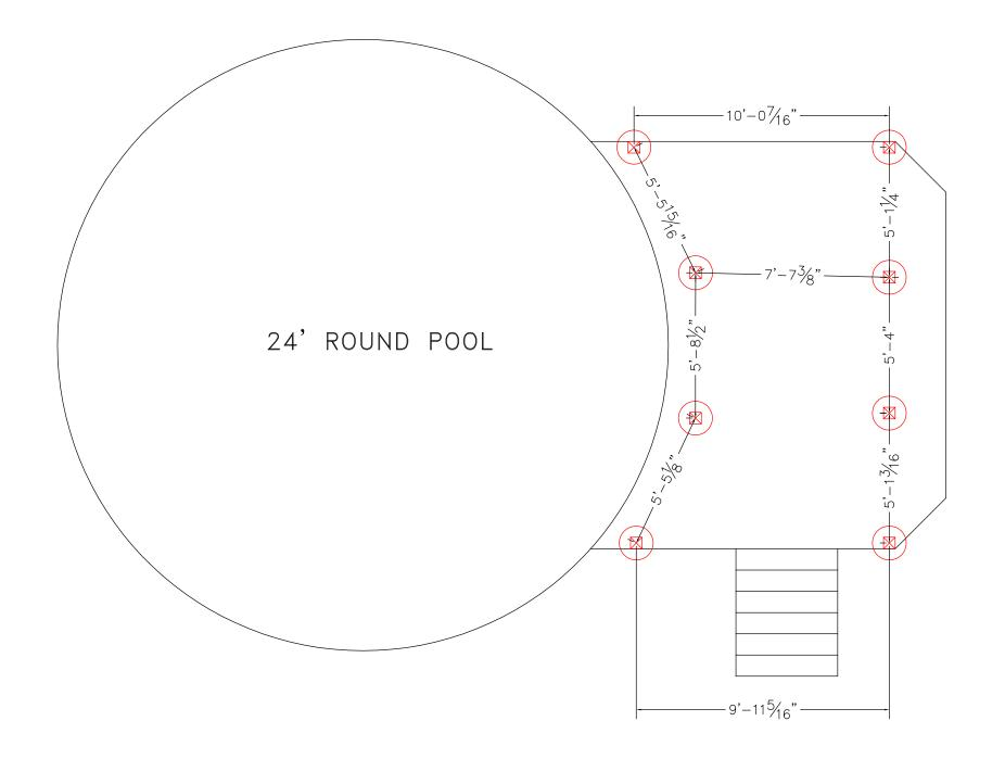
DISCLAIMER: USE ONLY 2,500 PSI CONCRETE FOR FROST FOOTING FOUNDATIONS
