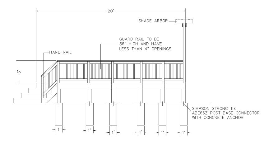
DISCLAIMER: ONLY USE #2 OR BETTER PRESSURE TREATED SOUTHERN YELLOW PINE 2 x 10 FOR FRAMING MATERIALS NEVER SUBSTITUTE COMPOSITE OR SOFTWOODS FOR FRAMING MATERIALS
