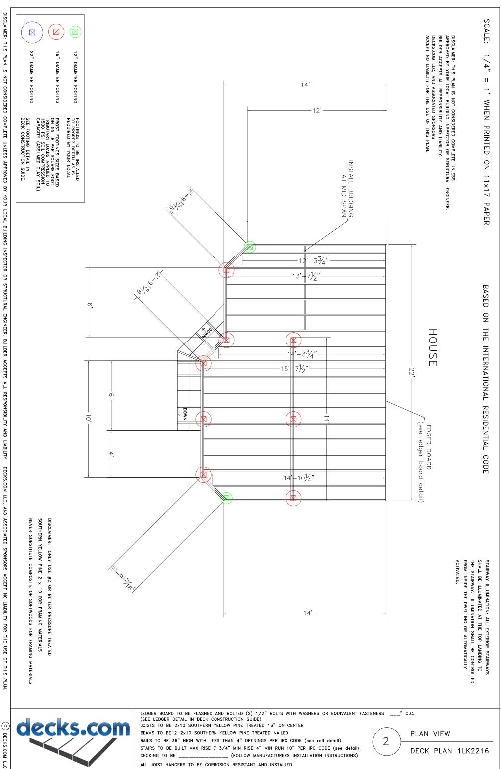
RAILS TO BE 36" HIGH WITH LESS THAN 4" OPENINGS PER IRC CODE (see rail detail) STAIRS TO BE BUILT MAX RISE 7 3/4" MIN RISE 4" MIN RUN 10" PER IRC CODE (see detail) DECKING TO BE \_\_\_\_\_ (FOLLOW MANUFACTURERS INSTALLATION INSTRUCTIONS)
