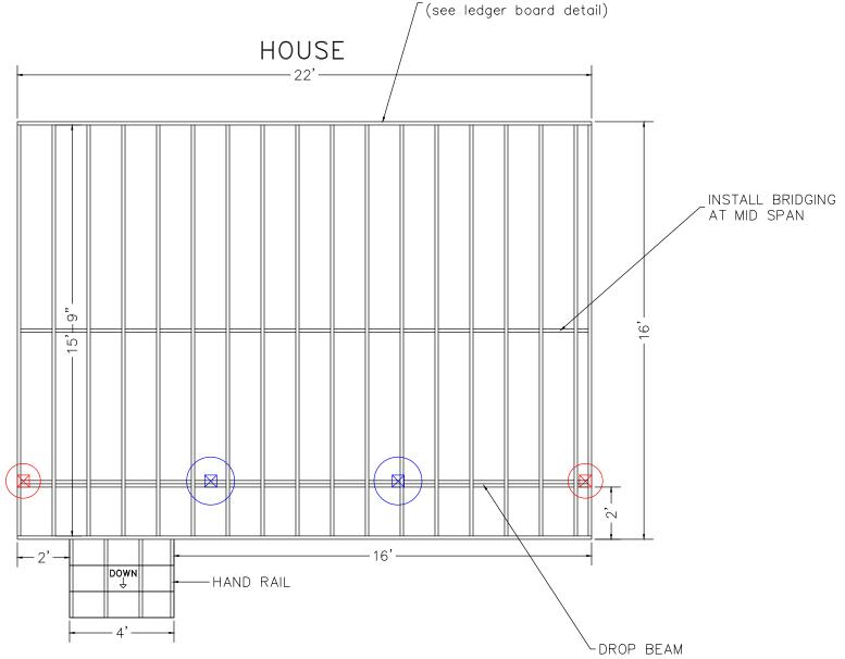
LEDGER BOARD TO BE FLASHED AND BOLTED (2) 1/2" BOLTS WITH WASHERS 16" O.C. (see led JOISTS TO BE 2x10 SOUTHERN YELLOW PINE TREATED 16" ON CENTER BEAMS TO BE 2-2x10 SOUTHERN YELLOW PINE TREATED NAILED RAILED RAILS TO BE 36" HIGH WITH LESS THAN 4" OPENINGS PER IRC CODE (see rail detail) STAIRS TO BE BUILT MAX RISE 7 3/4" MIN RISE 4" MIN RUN 10" PER IRC CODE (see detail)
