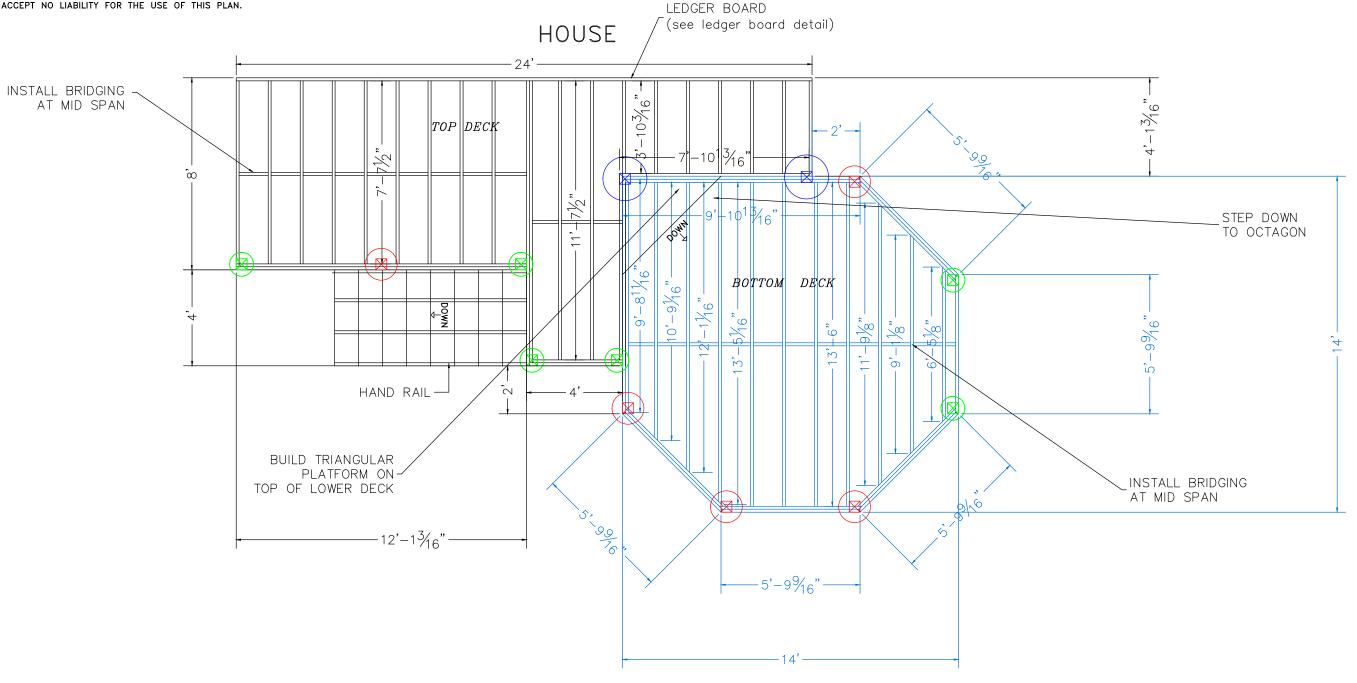
FOOTINGS TO BE INSTALLED TO PROPER DEPTH AS IS REQUIRED BY YOUR LOCAL 12" DIAMETER FOOTING BUILDING ORDINANCE
