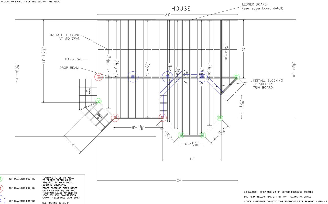
EDGER BOARD TO BE FLASHED AND BOLTED (2) 1/2" BOLTS WITH WASHERS OR EQUIVALENT FASTENERS — (SEE LEDGER DETAIL IN DECK CONSTRUCTION GUIDE)
