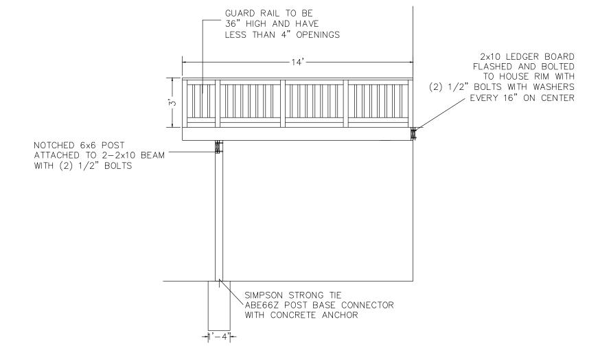
ROARD TO BE FLASHED AND BOLTED (2) 1/2" BOLTS WITH WASHERS OR EQUIVALENT FASTENERS
