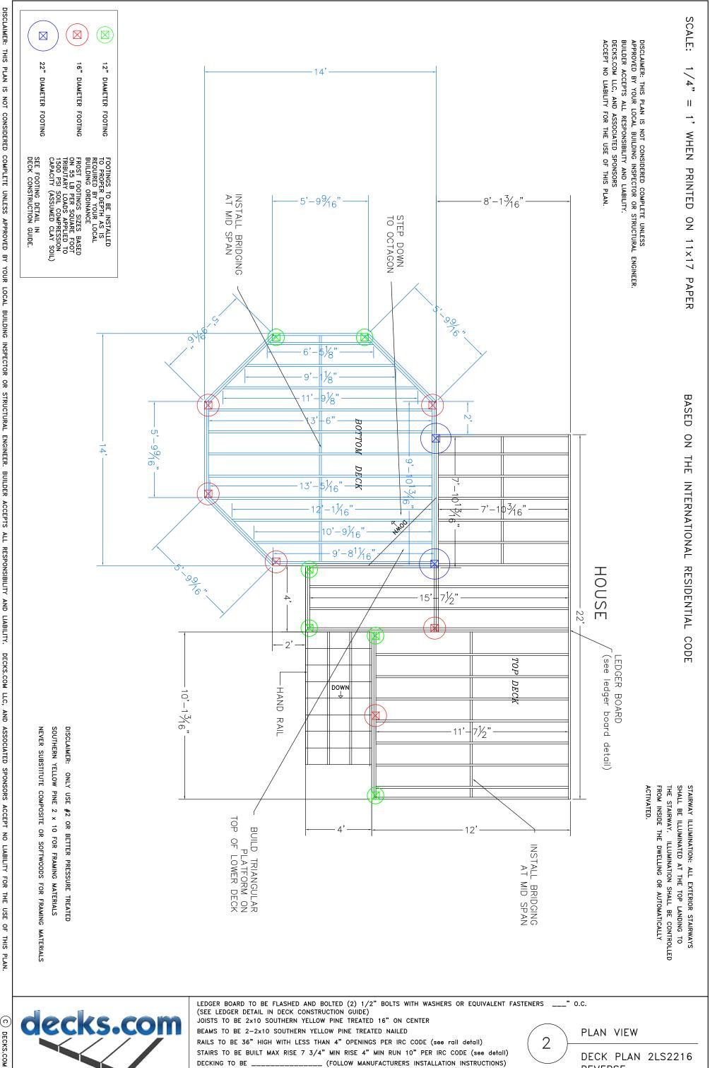
ALL JOIST HANGERS TO BE CORROSION RESISTANT AND INSTALLED
