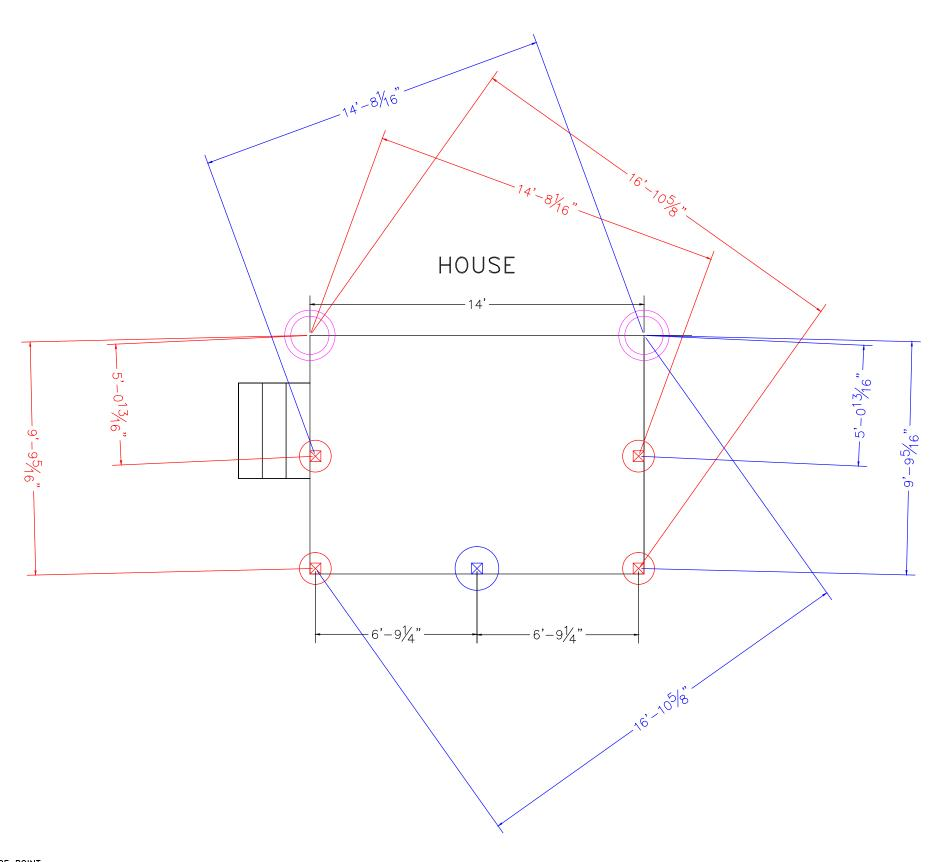
THIS IS A TRIANGULATION REFERENCE POINT MEASURE TO THE CENTER OF YOUR FOOTINGS FROM THESE POINTS. REFERENCE WWW.DECKS.COM/DECKBUILDING FOR MORE INFORMATION
