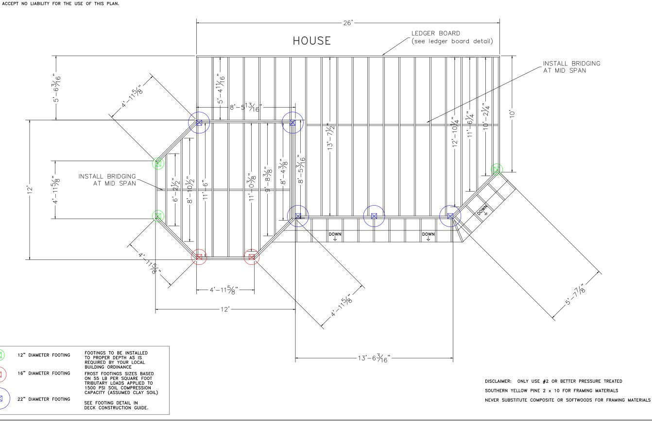
LEDGER BOARD TO BE FLASHED AND BOLTED (2) 1/2" BOLTS WITH WASHERS OR EQUIVALENT FASTENERS (SEE LEDGER DETAIL IN DECK CONSTRUCTION GUIDE)
