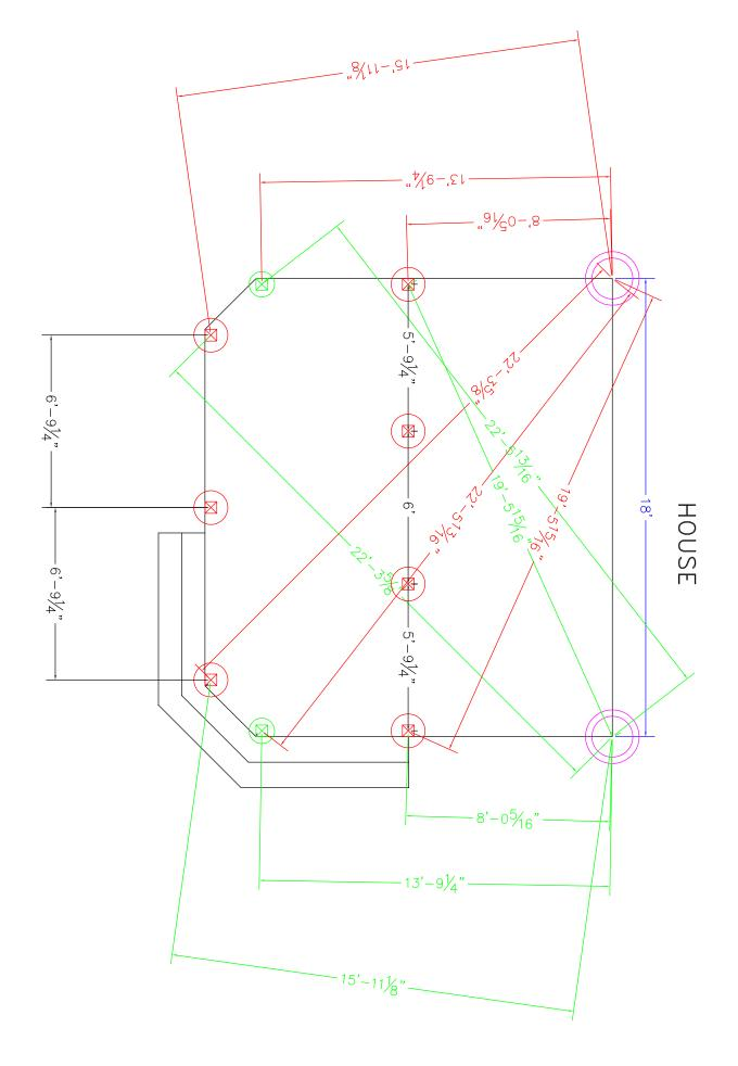
FOR FROST FOOTING FOUNDATIONS DISCLAIMER: USE ONLY 2,500 PSI CONCRETE
