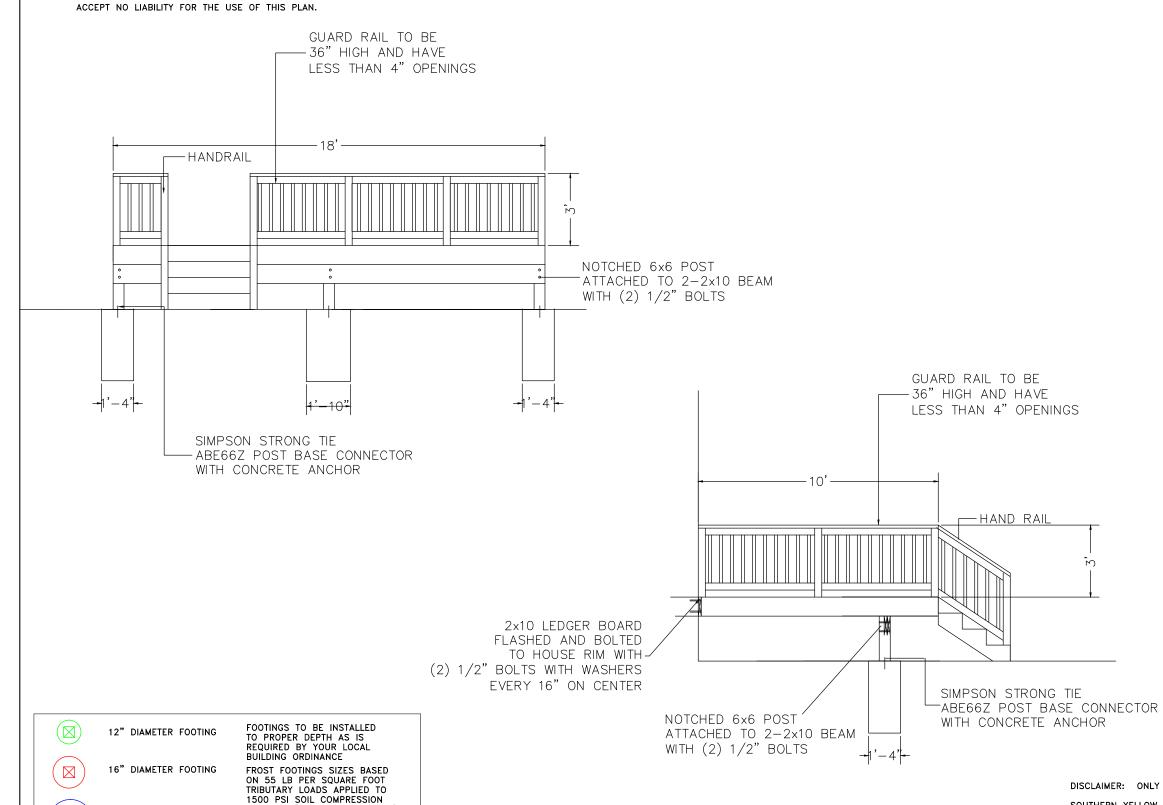
DISCLAIMER: ONLY USE #2 OR BETTER PRESSURE TREATED SOUTHERN YELLOW PINE 2 x 10 FOR FRAMING MATERIALS NEVER SUBSTITUTE COMPOSITE OR SOFTWOODS FOR FRAMING MATERIALS
