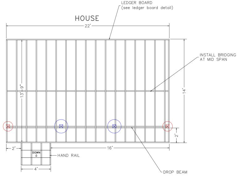
LEDGER BOARD TO BE FLASHED AND BOLTED (2) 1/2" BOLTS WITH WASHERS 16" O.C. JOISTS TO BE 2x10 SOUTHERN YELLOW PINE TREATED 16" ON CENTER BEAMS TO BE 2-2x10 SOUTHERN YELLOW PINE TREATED NAILED RAILS TO BE 36" HIGH WITH LESS THAN 4" OPENINGS PER IRC CODE (see rail detail) STAIRS TO BE BUILT MAX RISE 7 3/4" MIN RISE 4" MIN RUN 10" PER IRC CODE (see
