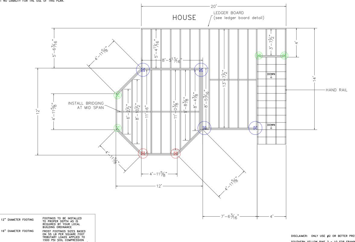
DISCLAIMER: ONLY USE #2 OR BETTER PRESSURE TREATED SOUTHERN YELLOW PINE 2 x 10 FOR FRAMING MATERIALS NEVER SUBSTITUTE COMPOSITE OR SOFTWOODS FOR FRAMING MATERIALS
