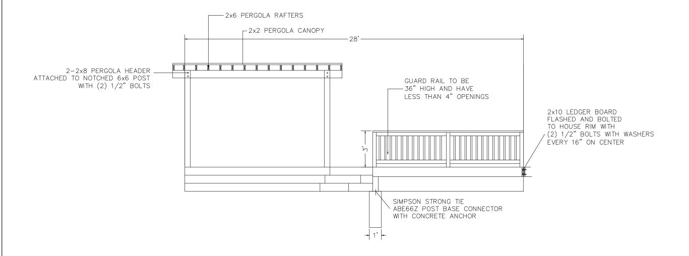
LEDGER BOARD TO BE FLASHED AND BOLTED (2) 1/2" BOLTS W (SEE LEDGER DETAIL IN DECK CONSTRUCTION GUIDE)
