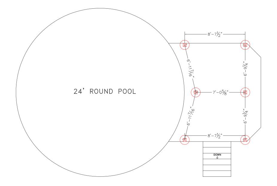
DISCLAIMER: USE ONLY 2,500 PSI CONCRETE FOR FROST FOOTING FOUNDATIONS
